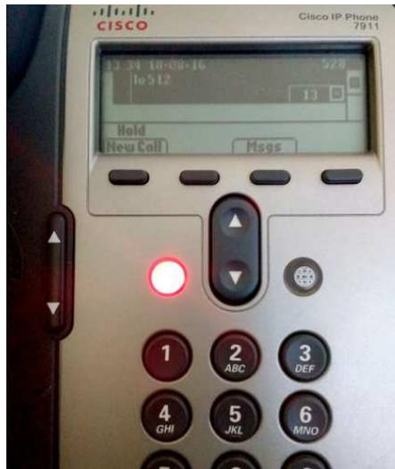
Whilst the incoming line remains on hold, dial-in the number to which you wish to transfer the call to. When the other line responds, you may transfer the line to the final destination by pressing the “Transfer” soft button
